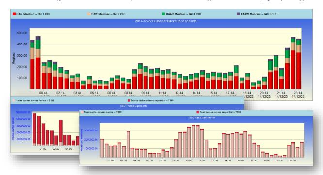
$6.\ DCOLLECT\ analysis\ shows\ the\ actual\ utilization\ rates\ of\ 3390\ disks,\ STO group\ SMS\ +\ optimization\ of\ Thin\ Provisioning.$
